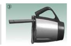
The measuring cup is a multi-purpose item: it is a closing cap for the hole in the mixing bowl lid to avoid heat loss and it prevents ingredients from escaping. The measuring cup can be used to measure ingredients. Besides the 100 ml mark please note that a measuring cup holds up to 100 ml, and 50 ml when filled to the notch. Place the measuring cup into the hole in the mixing bowl lid with its opening showing upwards ②.
